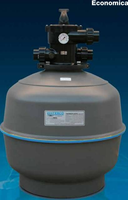
Thermoplastic granular filters operate on the basis of "depth filtration"; dirt is driven through the filter bed and trapped in minute spaces between the particles of filter media.
