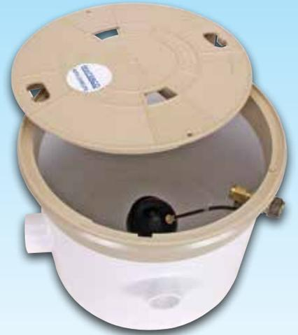
The Waterco Automatic Water Leveller is placed in the ground at a convenient location near the pool and plumbed to a separate pool inlet and also to the fresh water supply. The leveller remains inactive until the pool water level drops below or rises above the correct point at which time it will restore the right level by adding or draining water as the situation requires.
