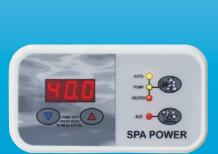
A simple, easy to use pool side touch pad with a digital readout and clearly labelled buttons to control pump on/off, heater on/off or auxillary pump on/off, water temperature setting and filtration time selection. The digital readout also shows pool water temperature and diagnostic error codes.
