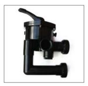
4. a. Assemble the MP Valve onto the tank by threading the unions onto the top and bottom tank connectors. Make sure the rubber Orings are in place in order to make the connections watertight.
