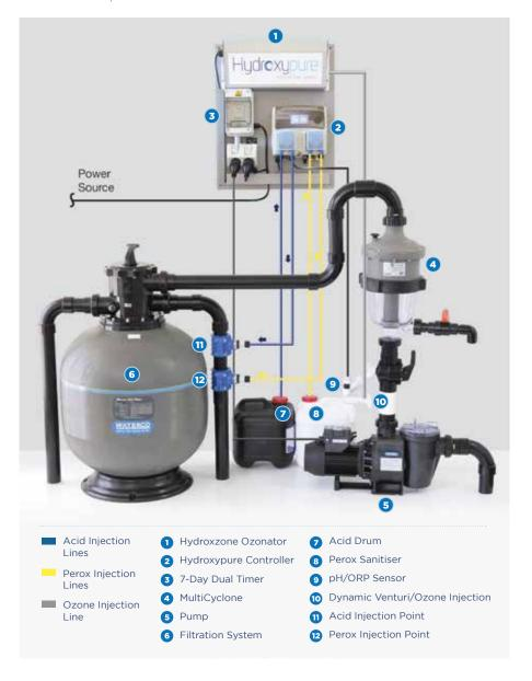
Pool water passes through a venturi (a tube that increases the water flow rate similar to a jet effect), which injects ozone into the water. The ozone then reacts with residual Perox in the water, producing a powerful oxidisation reaction.
