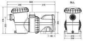
$<sup>^{\</sup>star}$  Suction & delivery accept 40mm PVC pipe on the I.D. and 50mm fitting on the O.D.
